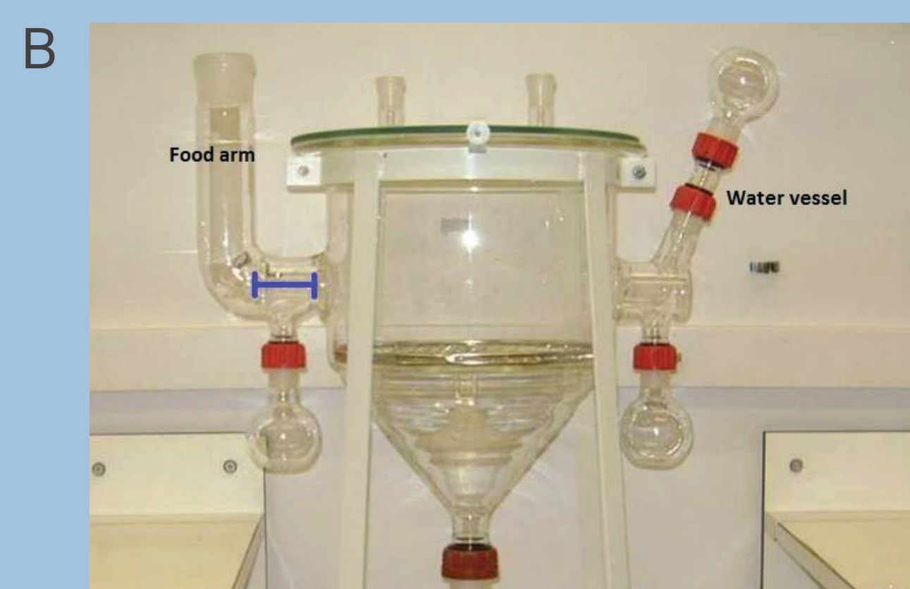
A) Typical Metabowl set-up for animals with tail exteriorisation. B) Example of amended Metabowl enabling easier access to food and water. C) Animal with nape of neck exteriorisation and harness attachment of swivel system.
