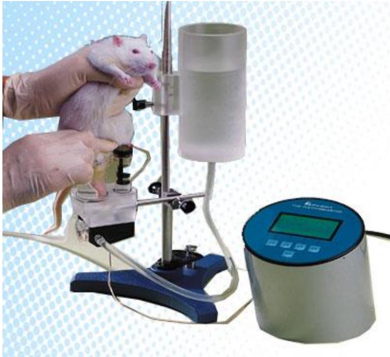
The Ugo Basile™ **Plethysmometer** is a microprocessor-controlled volume meter that has long been the standard instrument for measurement of rodent paw volume.
